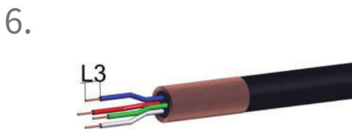
去除单线的介电绝缘层 (L3 = 4 mm [.157"])
