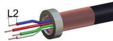
去除单线的介电绝缘层 (L2 = 4 mm [.157"])
