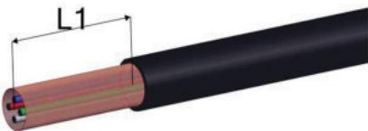
小心地去除电缆护套 (L1 = 28 mm [1.102"])
